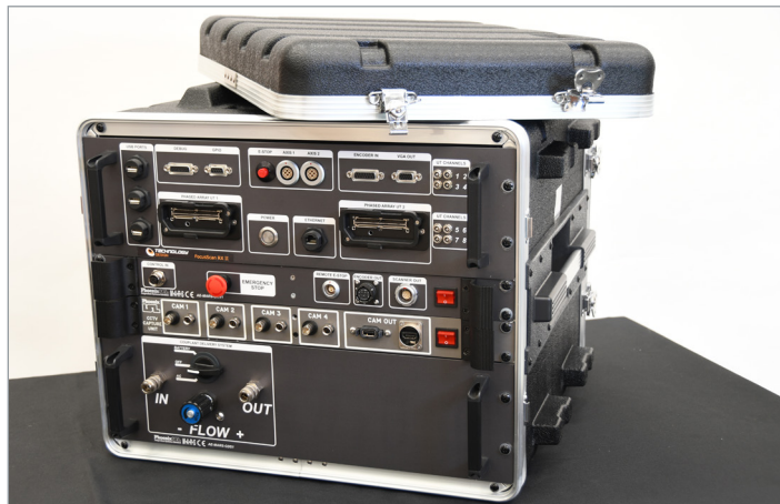
MARS Custom-Design Midi Rack System with Rack Mount FSRX II, Couplant Delivery System, Motor Controller and High Definition CCTV capture and lighting control.
