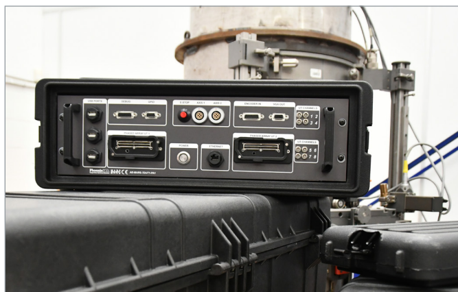
MARS Rack Mount FSRX II acquisition unit in transport case enclosure
