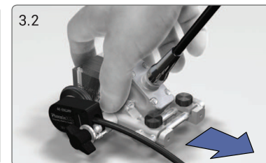
3.2 Scan forwards or backwards with the encoder mounted on the side
