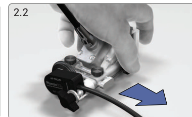
2.2 Scan left or right with the encoder mounted on the back
