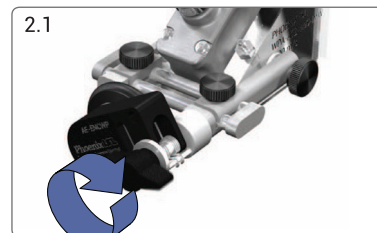
2.1 Screw on the encoder and set the spring tension
