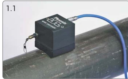
Magnetic encoder mount, attaches to 100mm OD to flat, ferritic material.
